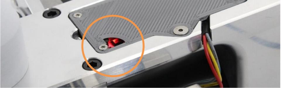
**Once you are sure there are no lights**, unplug the scale power cord and install the jumper wire as shown.
